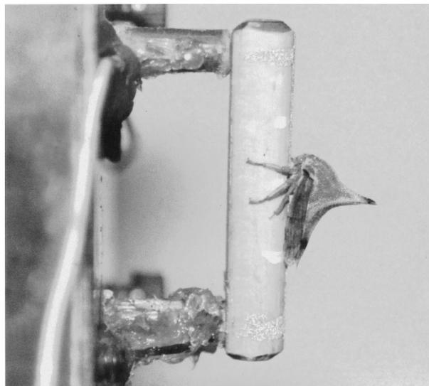
FIG. 1. *Umbonia crassicornis* (total length 10 mm) on the bending wave simulator. The insect's feet occupy a portion of the dowel (length 30 mm, diameter 6 mm) extending less than 1/8th the distance between the actuators in either direction from the middle. It is necessary to simulate a bending wave only over this narrow portion. From Cocroft *et al.* (2000), reprinted with permission.
