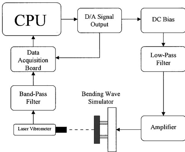
FIG. 2. Experimental setup for the bending wave simulator.
